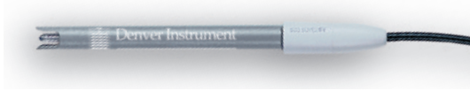
pH/ATC Epoxy-body Combination Electrode 300728.1 3M KCl liquid filled. BNC and 2.5 mm phone plug connector. Standard on Denver Basic Meter.
