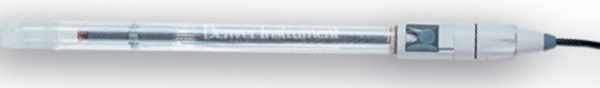
High-Performance Sleeve-Junction Combination Electrode 300738.1 3M KCl liquid filled with BNC. For non-aqueous or low ionic strength samples
