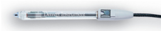
pH/ATC Glass-body Combination Electrode 300729.1 3M KCl liquid filled. BNC and 2.5 mm phone plug connector. Standard on Denver 200 series and Basic-Bio Meter. TRIS buffer compatible.
