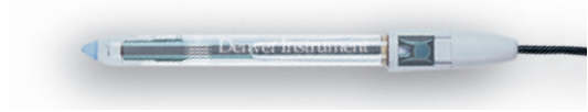
Glass-body Combination Electrode 300731.1 3M KCl liquid filled with BNC connector. Tris buffer compatible.
